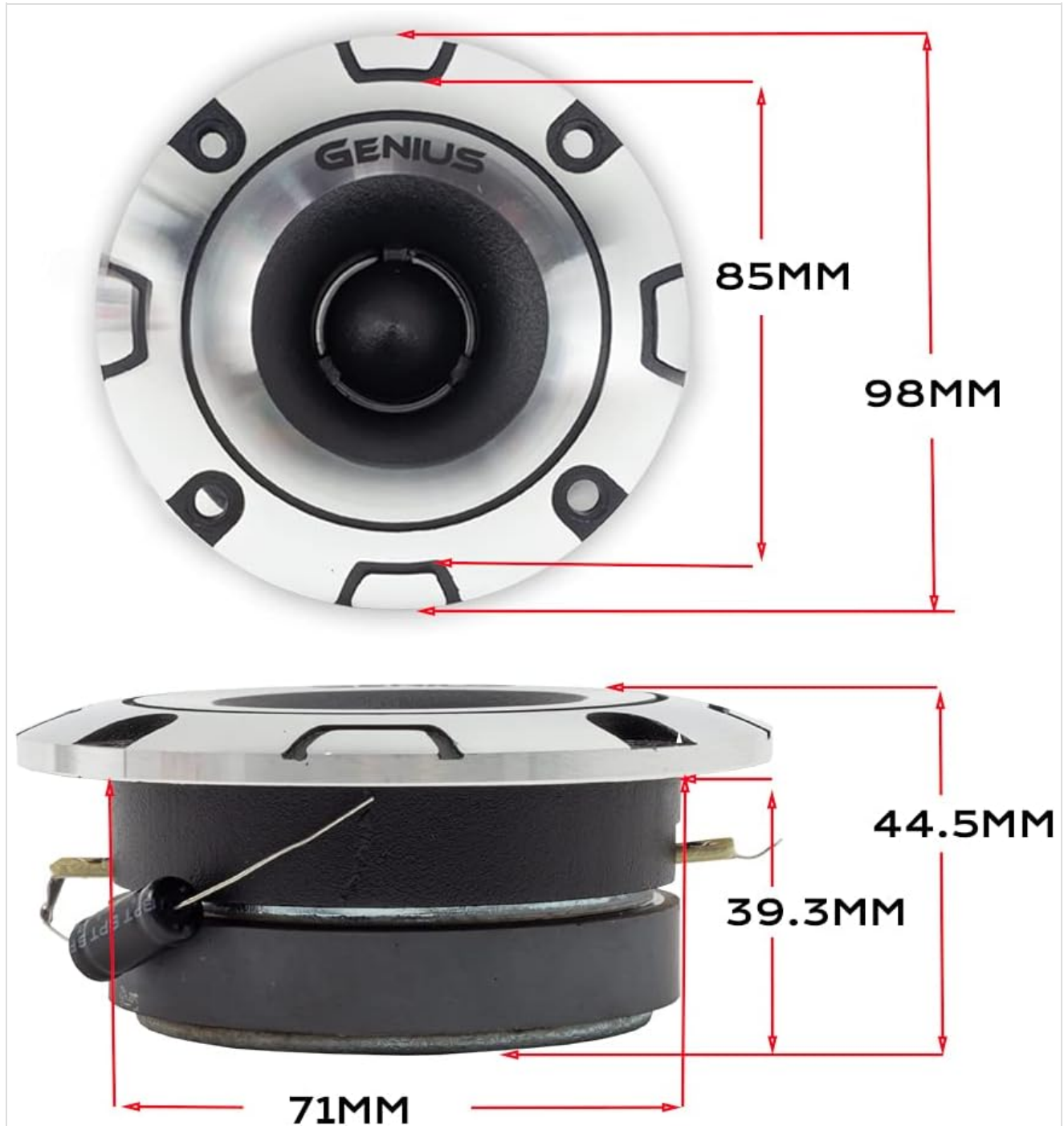
Image: Detailed dimensions of the GPRO-T08 tweeter for mounting reference.
