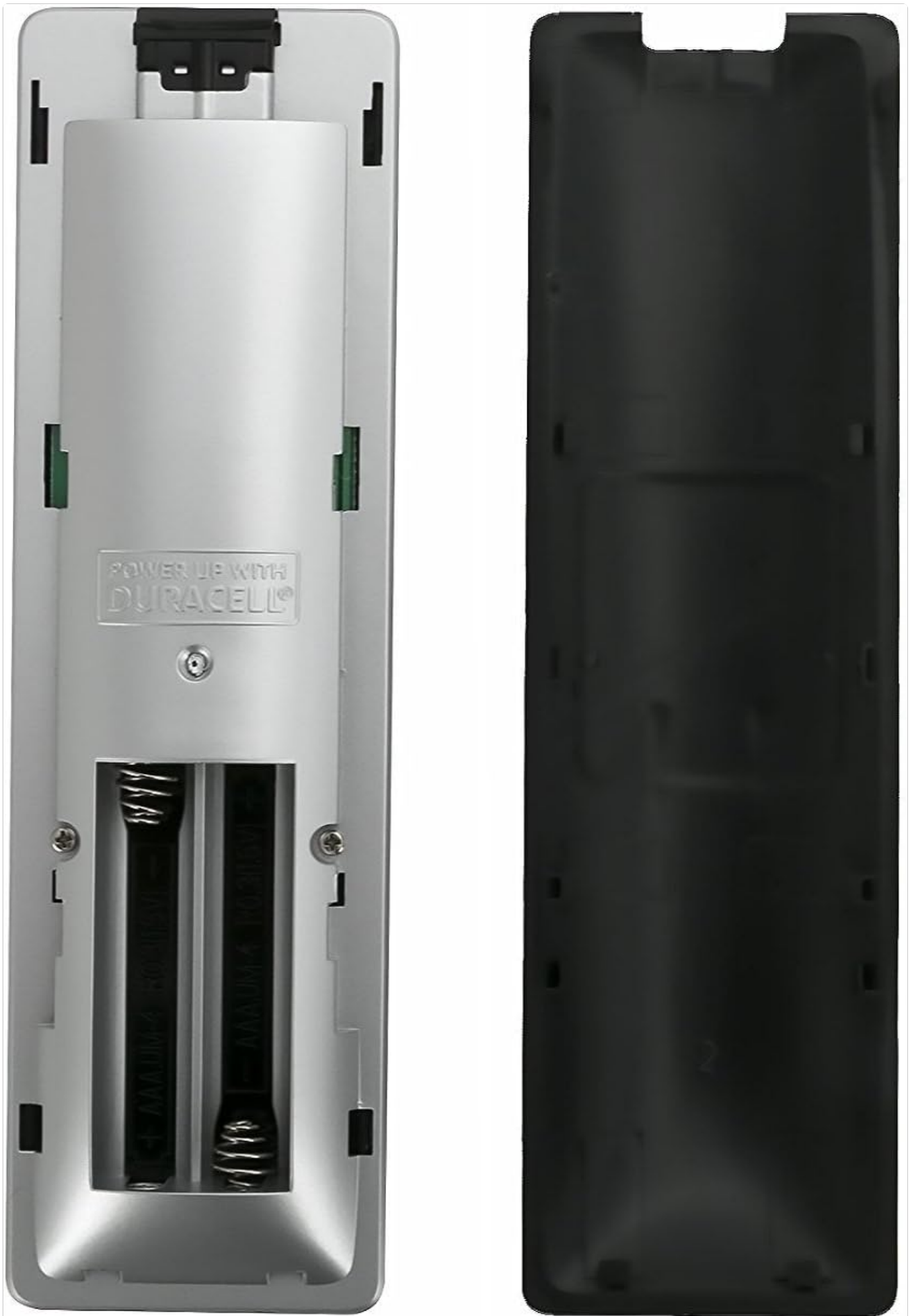
This image shows the back of the UBay XRS331-C remote control with the battery compartment open. It illustrates where to insert two AAA batteries, which are required for operation.
