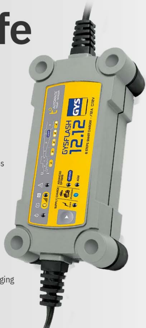
Figure 2.1: The GYSFLASH 12.12 charger is designed with multiple safety features, including IP65 protection against dust and water, an integrated temperature probe to prevent overheating, and safeguards against electrical hazards such as polarity reversal, sparks, and overcharging.
