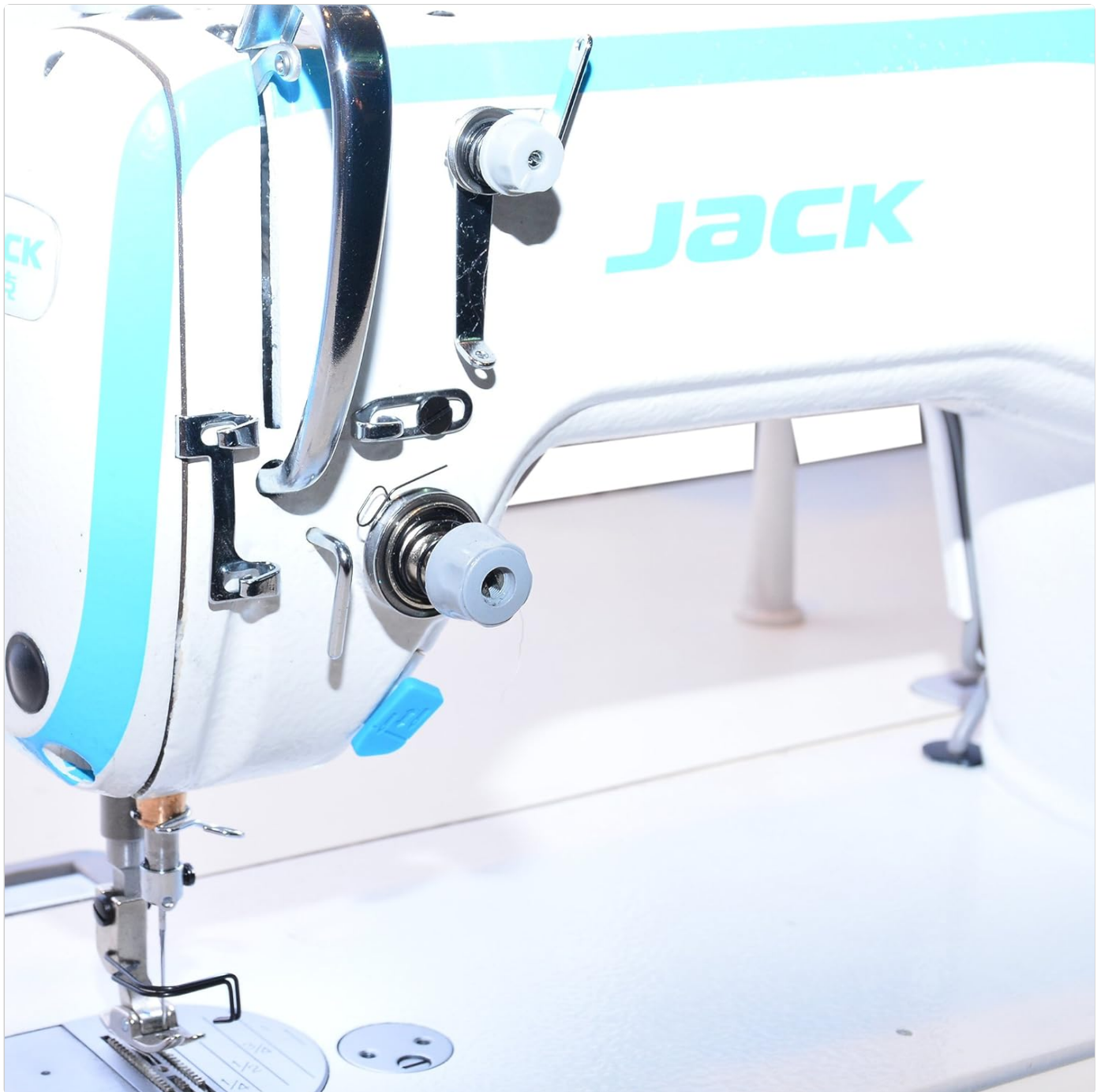
Figure 5: Close-up of the needle area, presser foot, and thread tension assembly on the Jack A2 sewing machine, showing the path of the upper thread.
