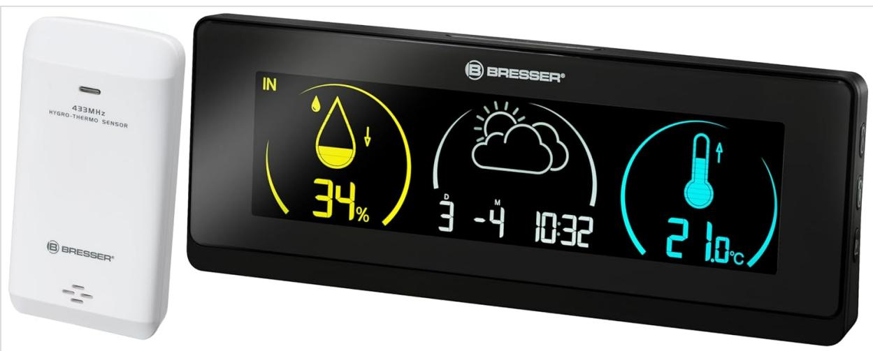
The compact outdoor sensor measures external temperature and humidity. It transmits data wirelessly to the main unit. The sensor requires 2x AA batteries (not included).
