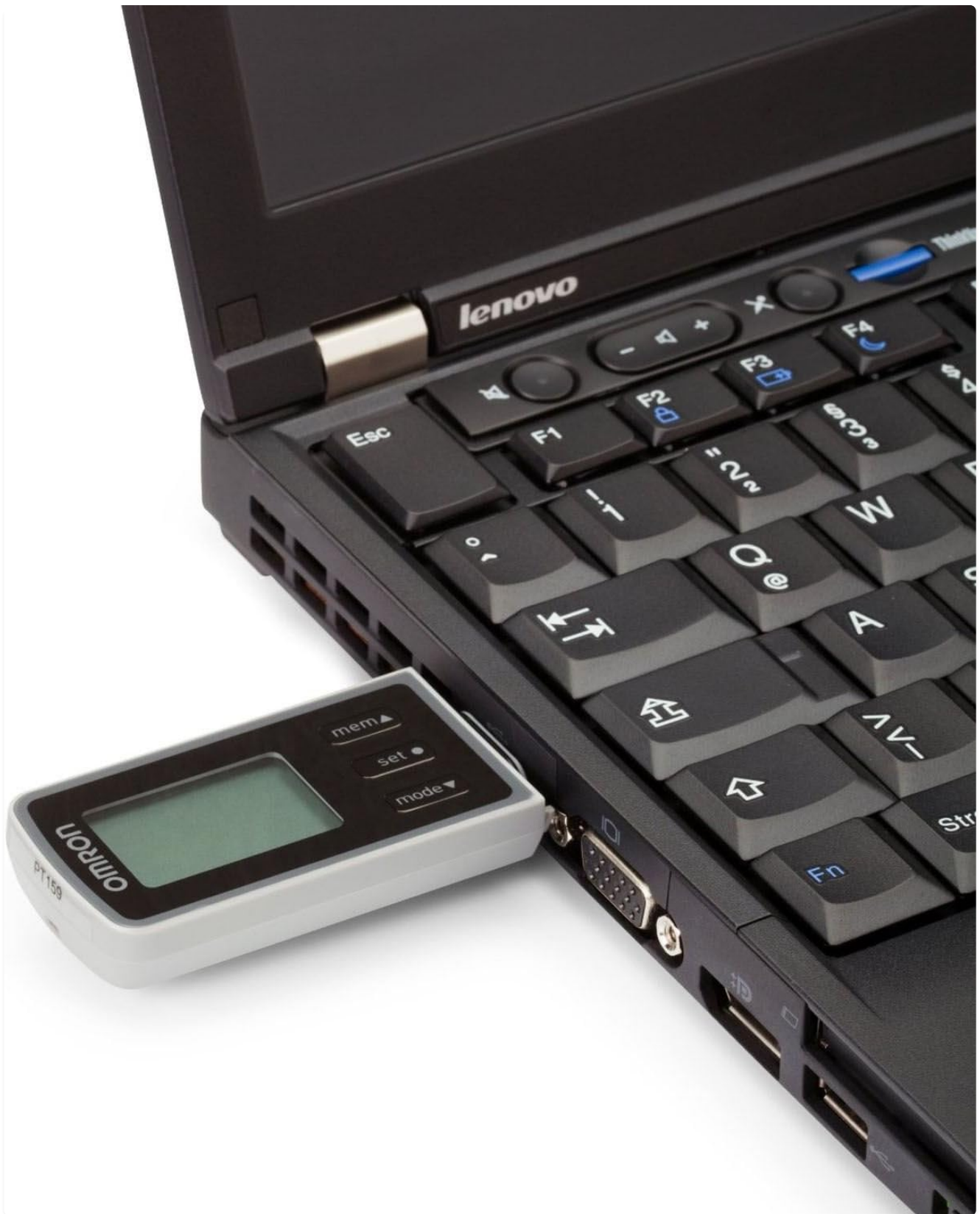
Figure 3: The Omron HJ322U-E Pedometer connected to a laptop, illustrating the data transfer capability via a USB dongle.
