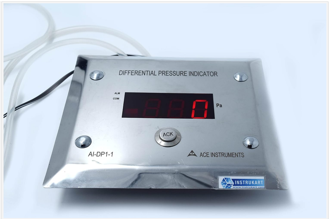
Figure 5: The AI-DP1-LED display showing a zero reading, indicating no differential pressure.
