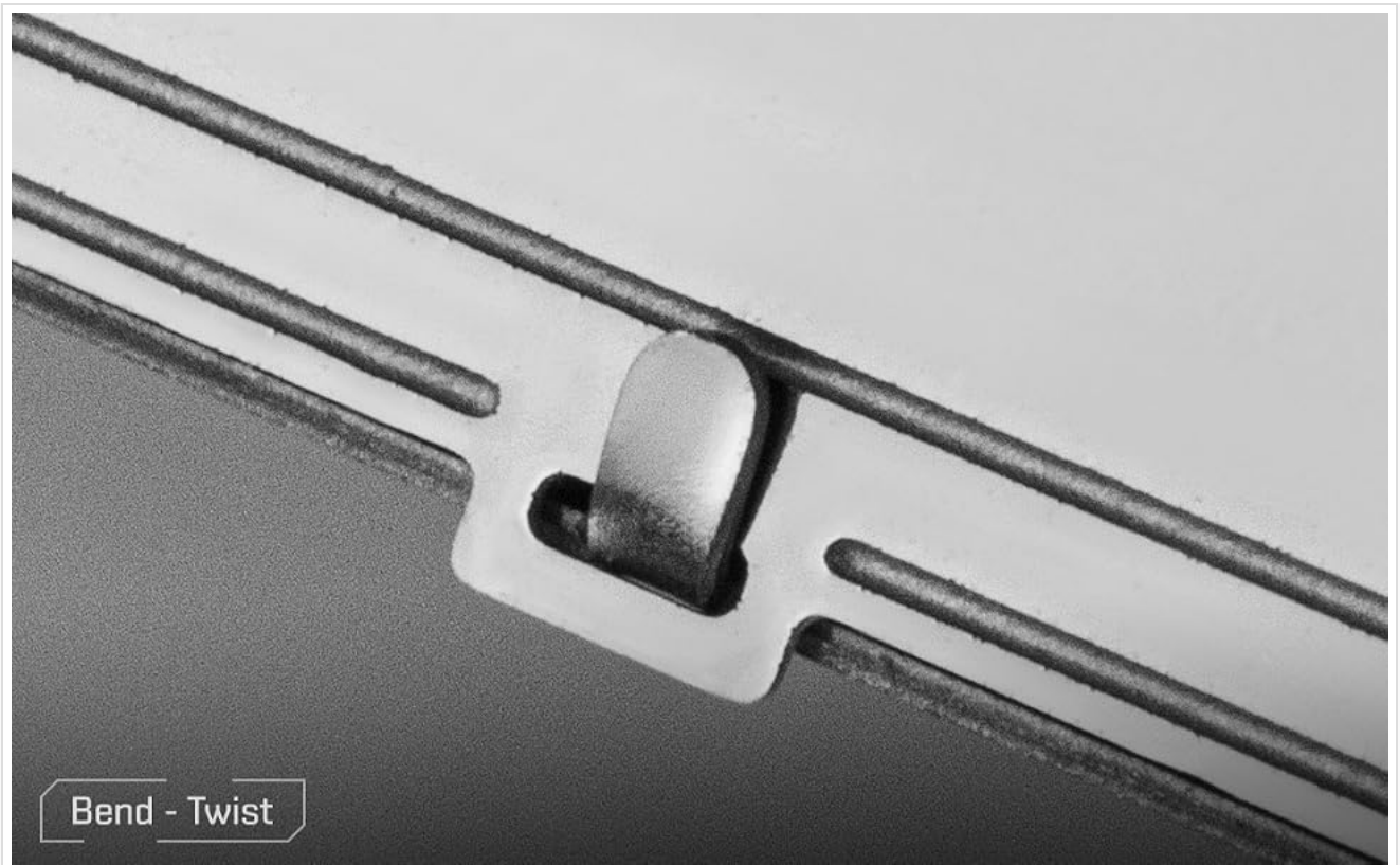
Image: A close-up demonstrating the 'Bend - Twist' method to secure a metal tab after insertion.
