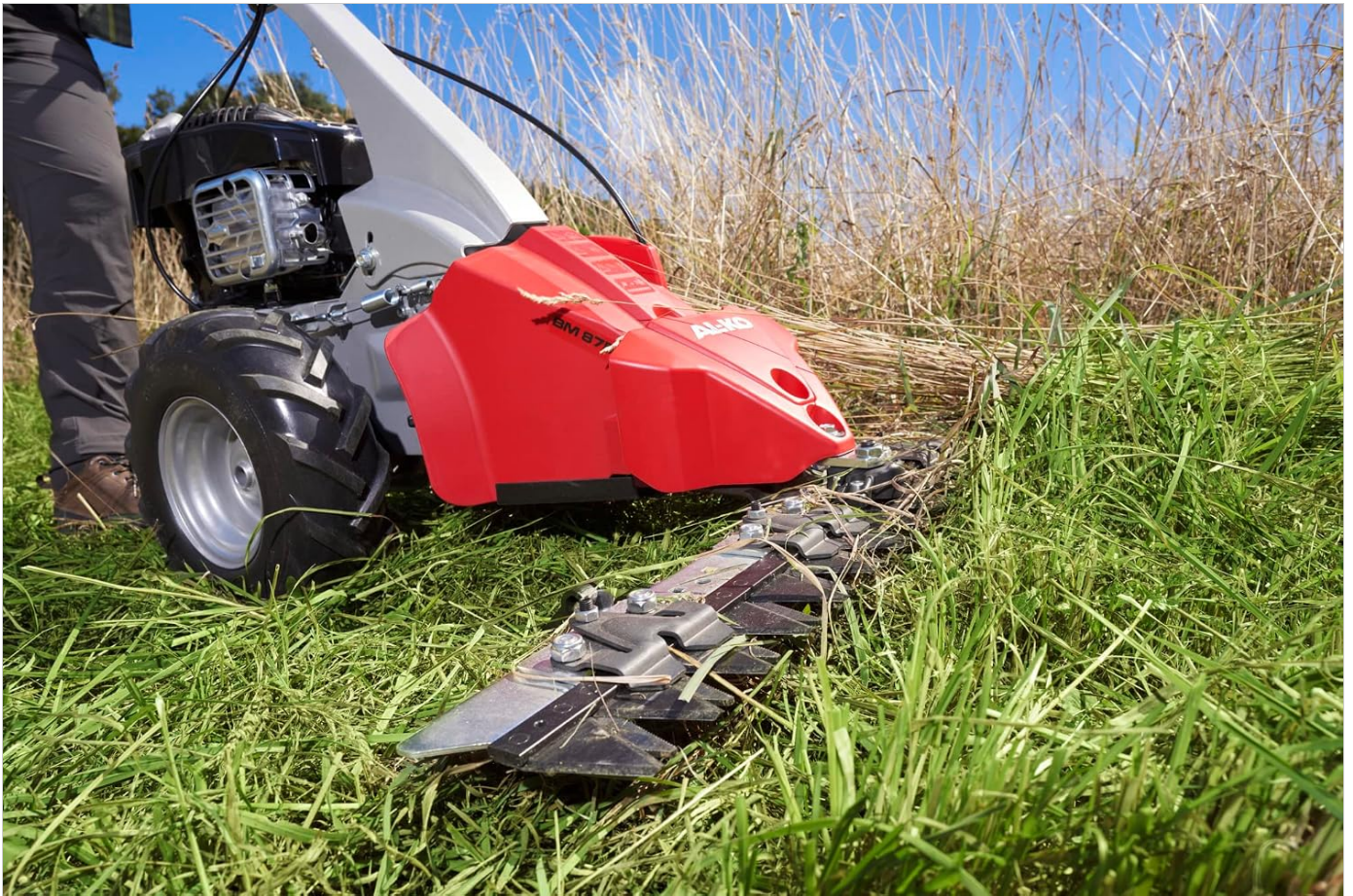
Figure 5.2: The ESM cutting bar efficiently cuts through dense vegetation. Ensure the cutting bar is clear of debris.
