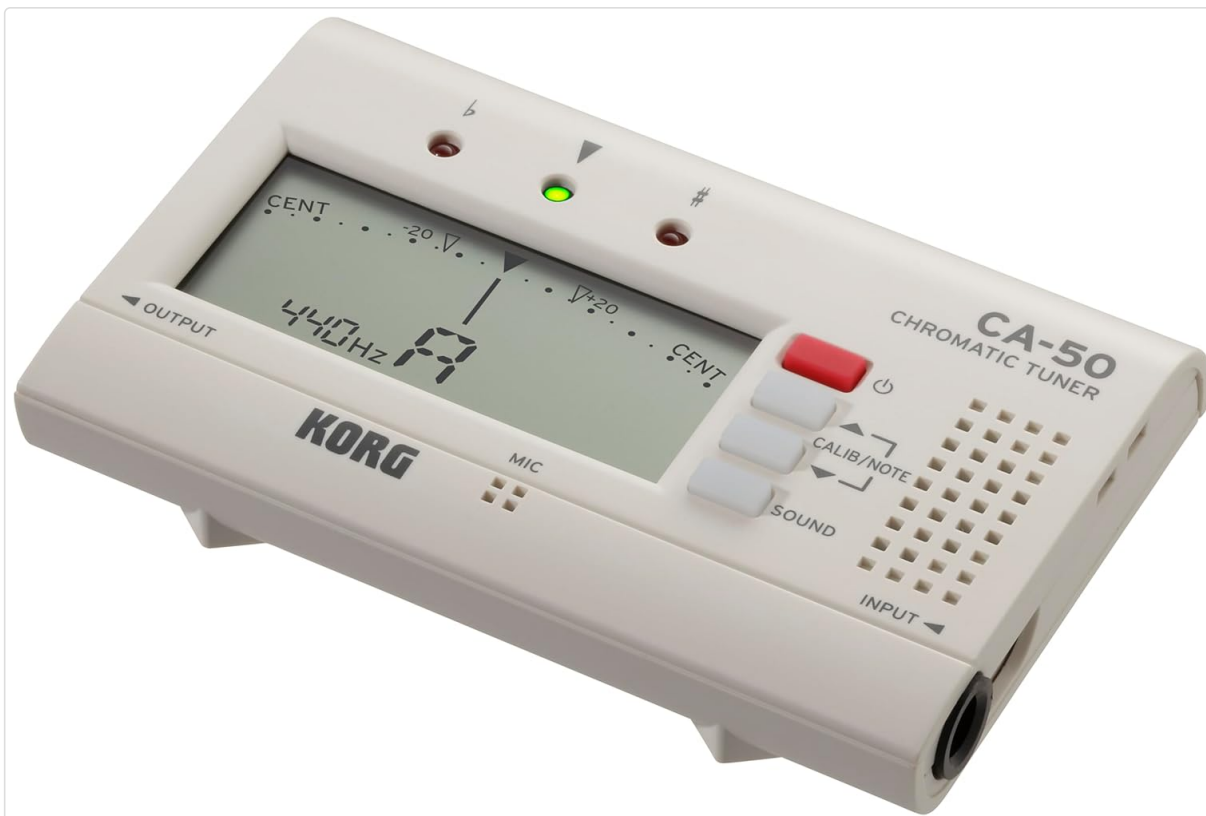
Figure 1: Front view of the Korg CA-50 Chromatic Tuner, showing the display, controls, and microphone.
