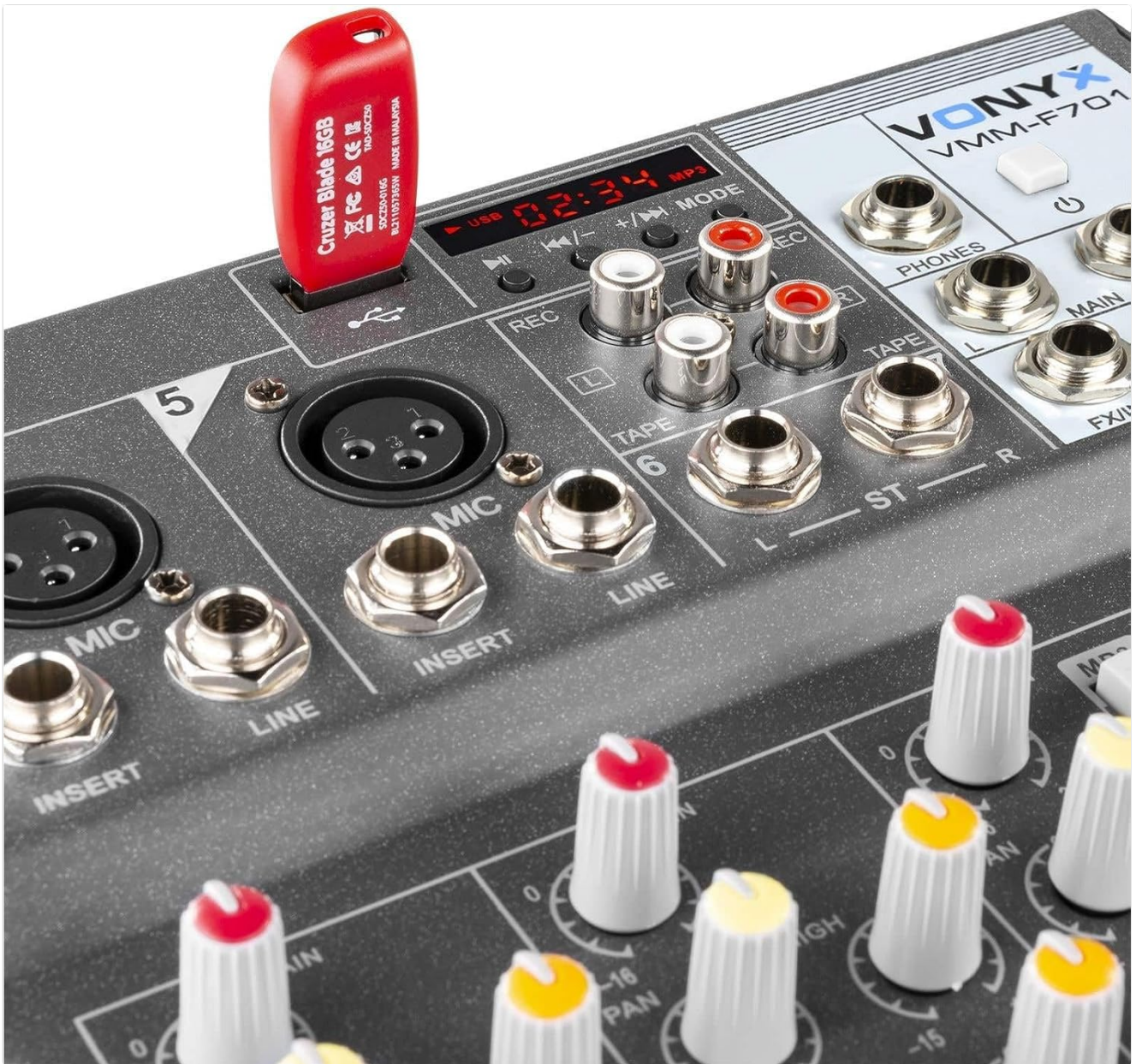
Close-up of the USB input and media player controls on the Vonyx VMM-F701 mixer, with a USB drive inserted.
