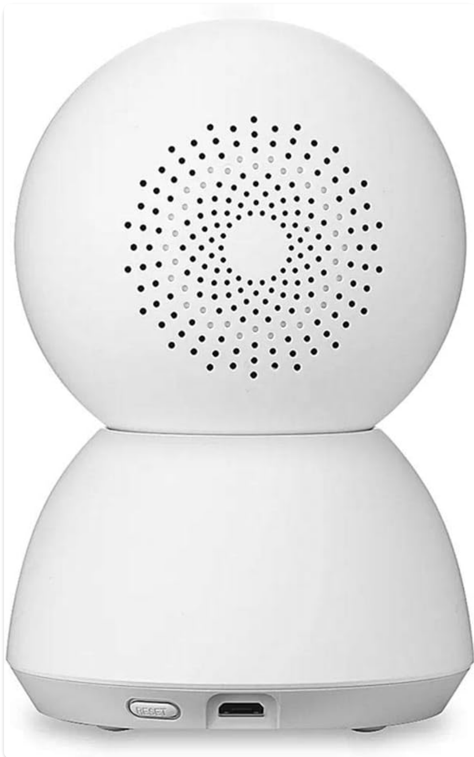
Image: Rear view of the Xiaomi Mi Home Security Camera, highlighting the reset button and the micro USB power input port.
