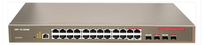
This image displays the front panel of the IP-COM G3224P switch. On the left, the IP-COM logo and model number G3224P are visible. To the right, there are LED indicators for SYS, PoE MAX, and individual port status. A console port is also present. The main section features 24 Gigabit Ethernet RJ45 ports, arranged in two rows, with port numbers 1 through 24. On the far right, there are four SFP ports labeled SFP1, SFP2, SFP3, and SFP4, which are used for fiber optic uplinks.
