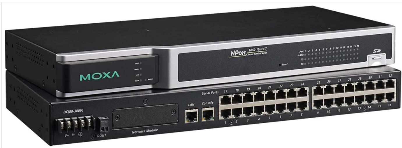
Figure 1: Front and rear view of the MOXA NPort 6650-16 Secure Device Server. The top unit shows the front panel with MOXA branding, status LEDs (PWR, Ready, Link, Alarm), a Reset button, and an SD card slot. The bottom unit shows the rear panel with DC power input (88-300V), a Network Module slot, DOUT, two LAN ports, a Console port, and 16 serial ports (numbered 17-32 on the top row, and 1-16 on the bottom row).
