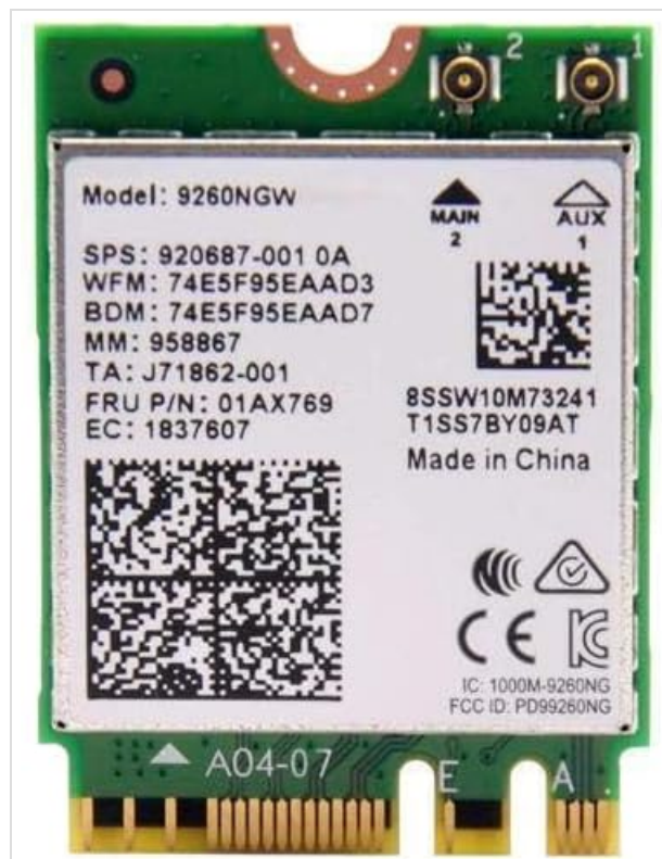
Figure 1: Intel Wireless AC 9260 M.2 network adapter. This image displays the compact M.2 form factor card, highlighting the two antenna connectors labeled 'MAIN' (2) and 'AUX' (1), the model number '9260NGW', and various regulatory compliance markings. The M.2 E-key interface is visible at the bottom.
