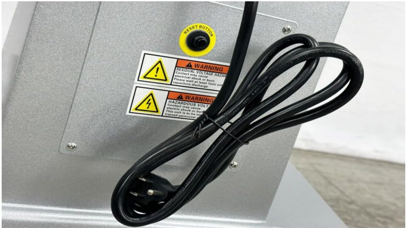
Figure 7: Bowl lift handle and the yellow reset button for thermal overload protection.
