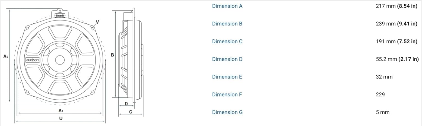
Figure 8.1: Technical drawing illustrating the dimensions of the Audison AP BMW S8-2 subwoofer. This diagram provides precise measurements for installation planning.
