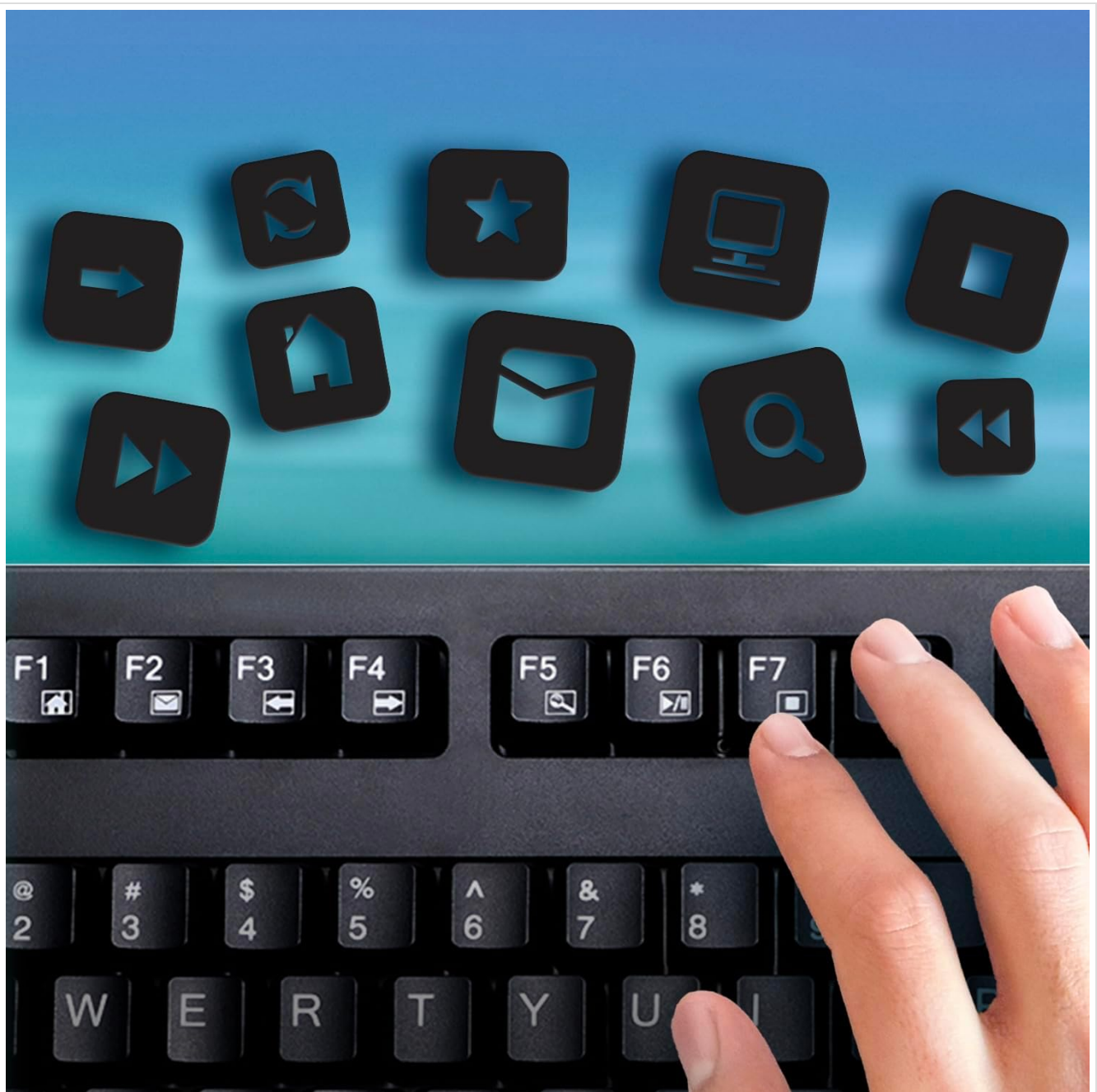
Figure 4: Detail of the multimedia and internet hotkeys located above the function keys, providing quick access to common controls.
