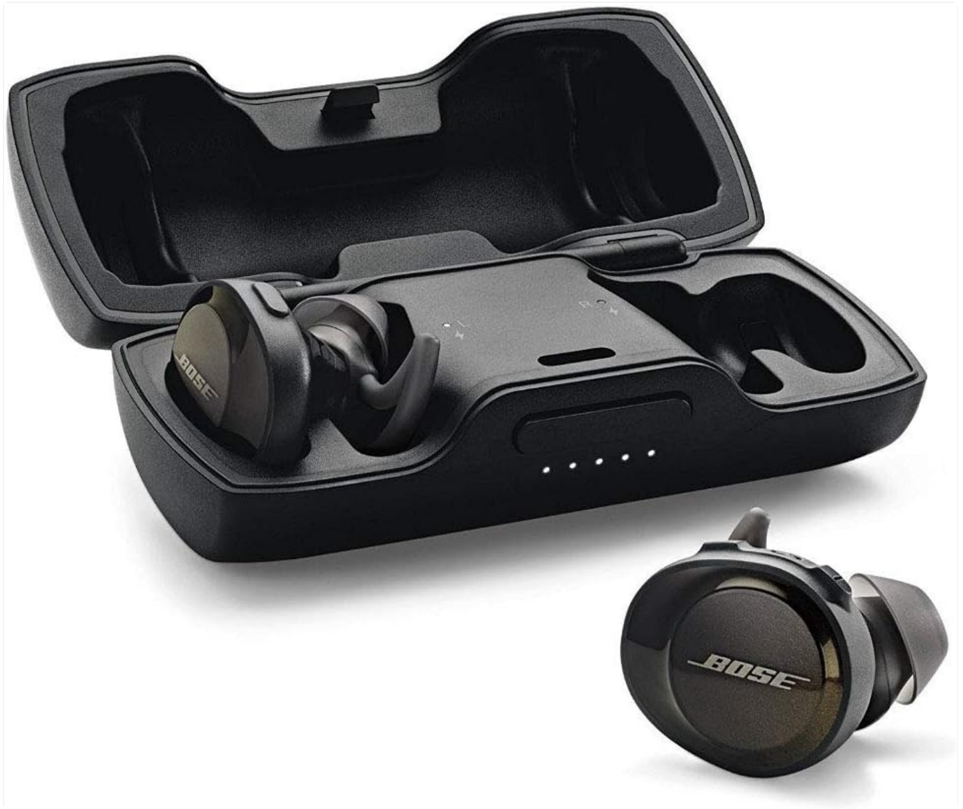
Figure 2: Earbuds charging within the portable charging case. The LED indicators on the case show the current battery level.
