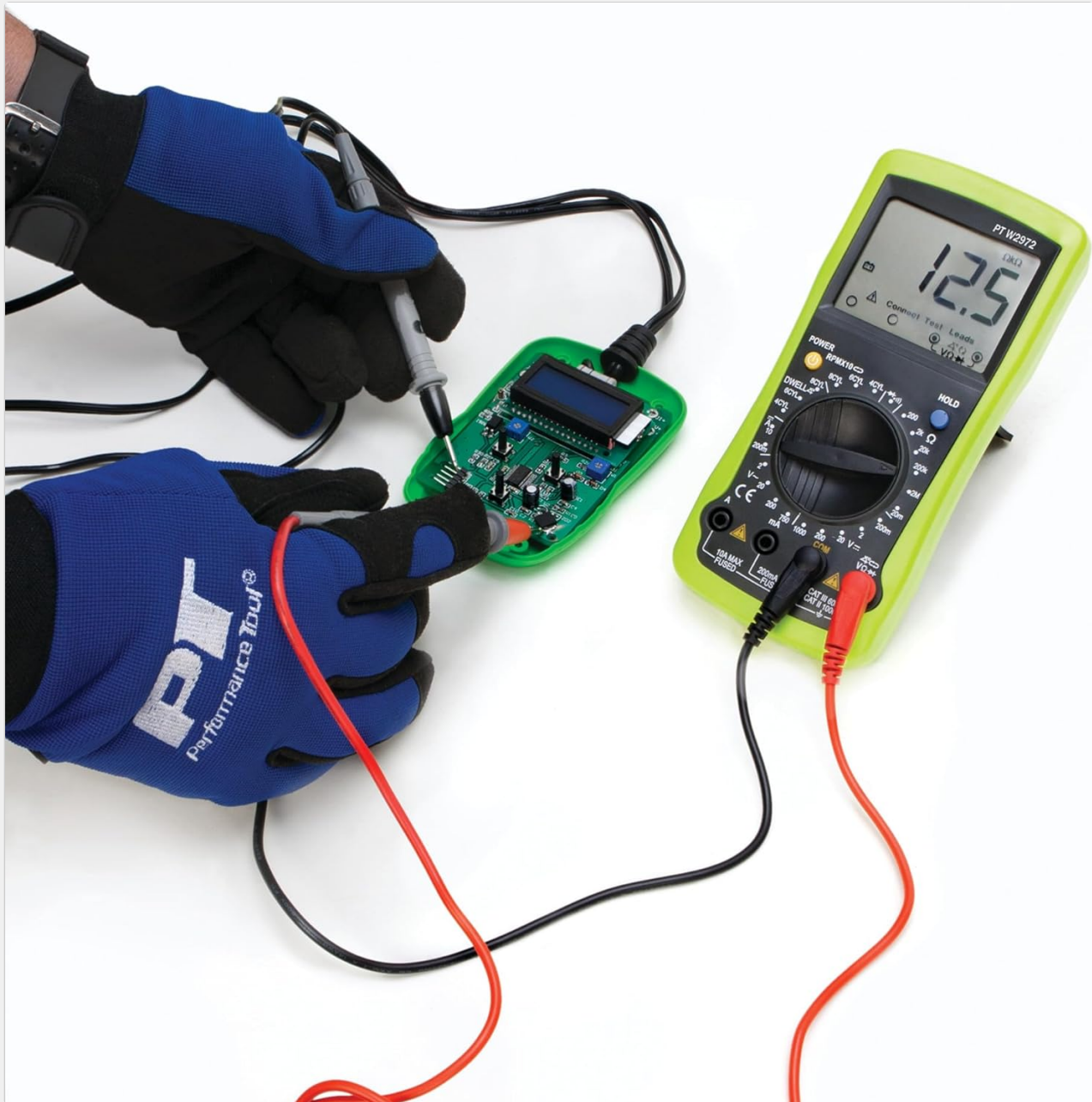
Image Description: A Performance Tool W2972 Multimeter displaying a resistance reading while connected to a small green circuit board. A person wearing blue gloves is using the test probes.
