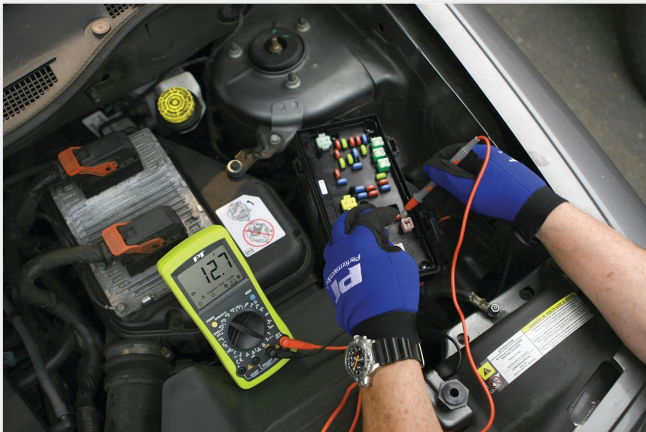
Image Description: A Performance Tool W2972 Multimeter displaying a voltage reading while connected to a car battery in an engine bay. A person wearing blue gloves is using the test probes.
