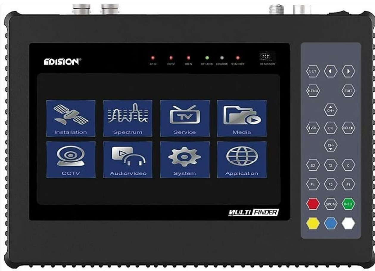
Image: The main menu interface of the EDISION MULTI-FINDER, displaying icons for different functions including Installation, Spectrum, Service, Media, CCTV, Audio/Video, System, and Application, allowing users to navigate to desired features.
