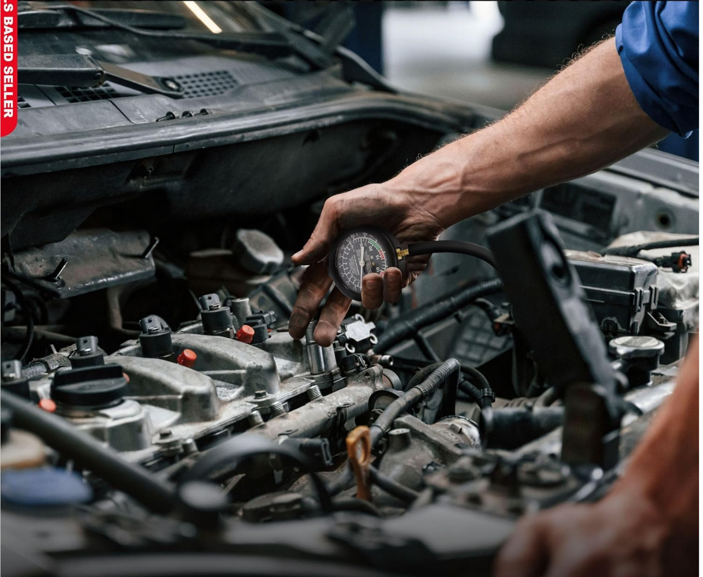
Figure 5.1: Performing a vacuum test on a vehicle engine.
