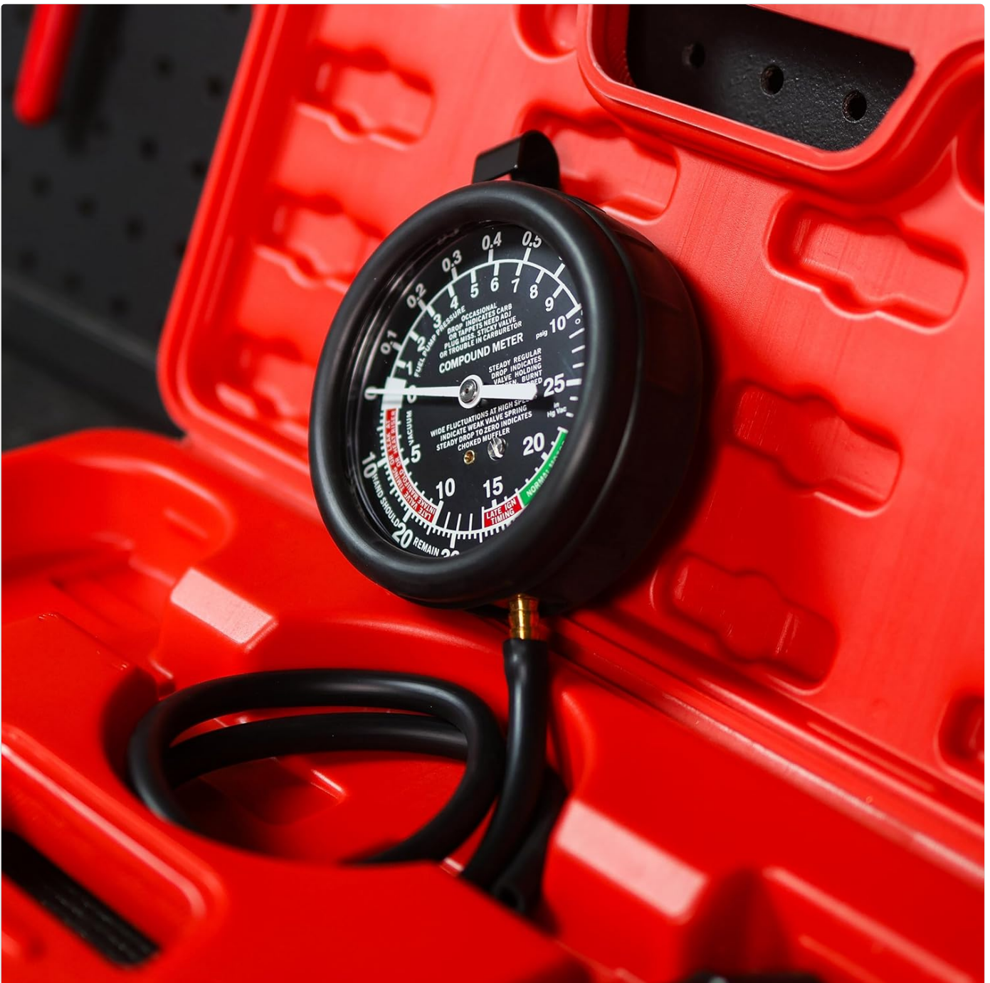
Figure 4.1: The gauge and hose ready for connection within the case.
