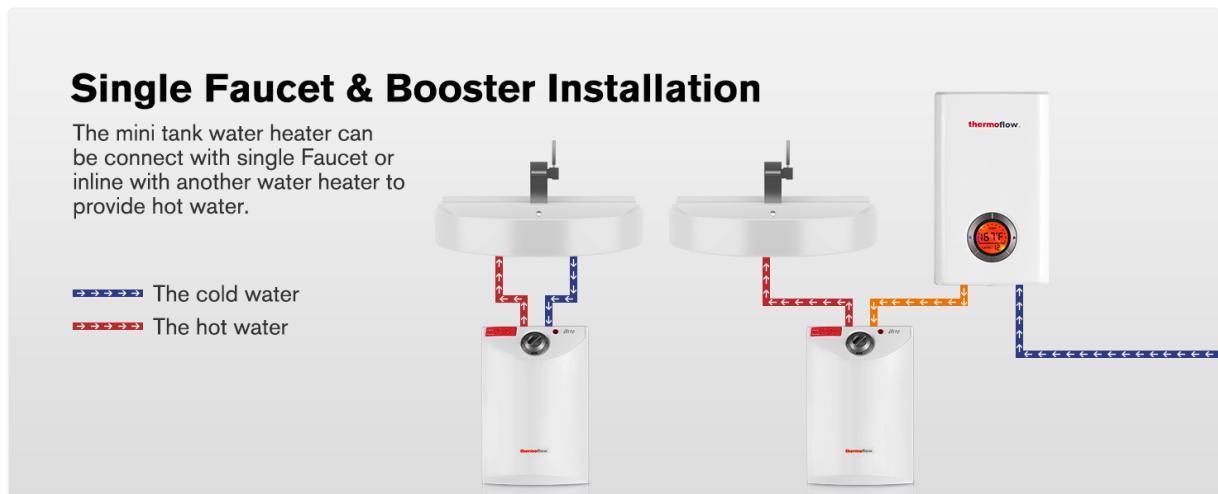
Image: Plumbing diagrams for connecting the mini tank water heater to a single faucet or in a booster configuration with an existing water heater.
