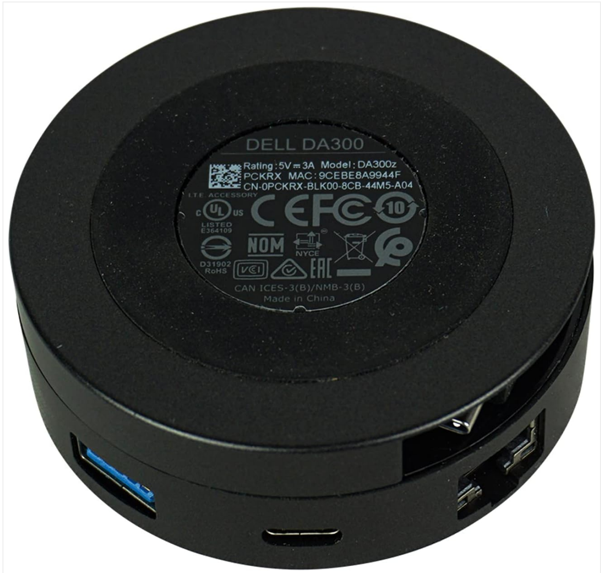
Figure 3: Bottom of the Dell DA300 adapter, displaying model number and regulatory compliance information.
