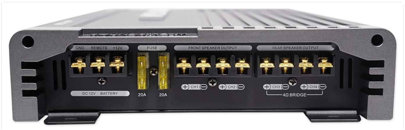
Image: The rear panel of the Soundstream AR4.1200 amplifier, showing the power, ground, remote, fuse, and speaker output terminals.
