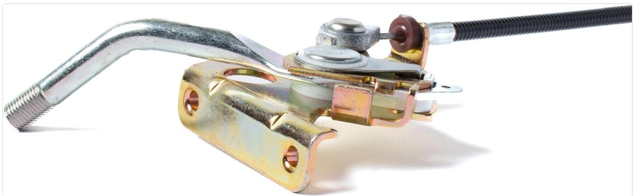
Figure 3: Angled view of the throttle cable assembly, showing the cable entry and lever components.
