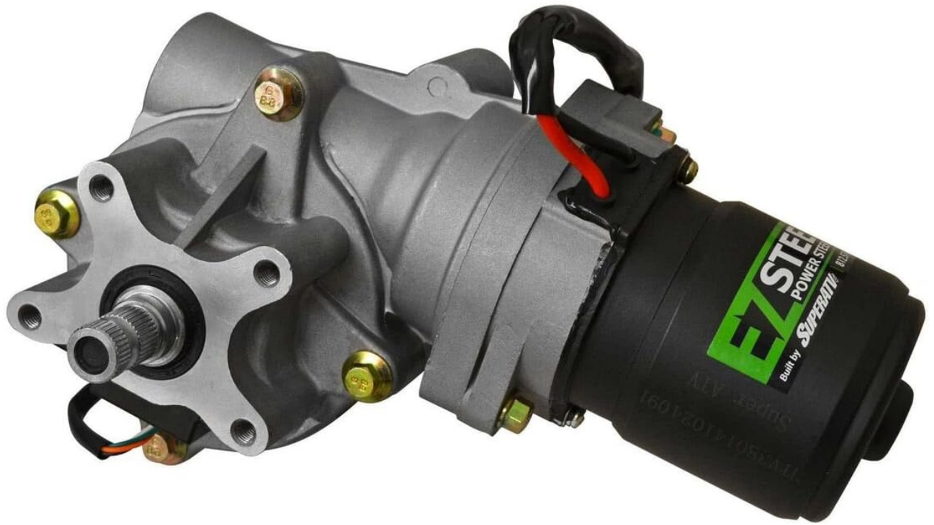
Figure 2.1: The powerful 380 Watt motor, central to the power steering system.
