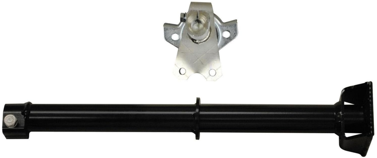
Figure 2.4: The steering shaft and associated components for integration.
