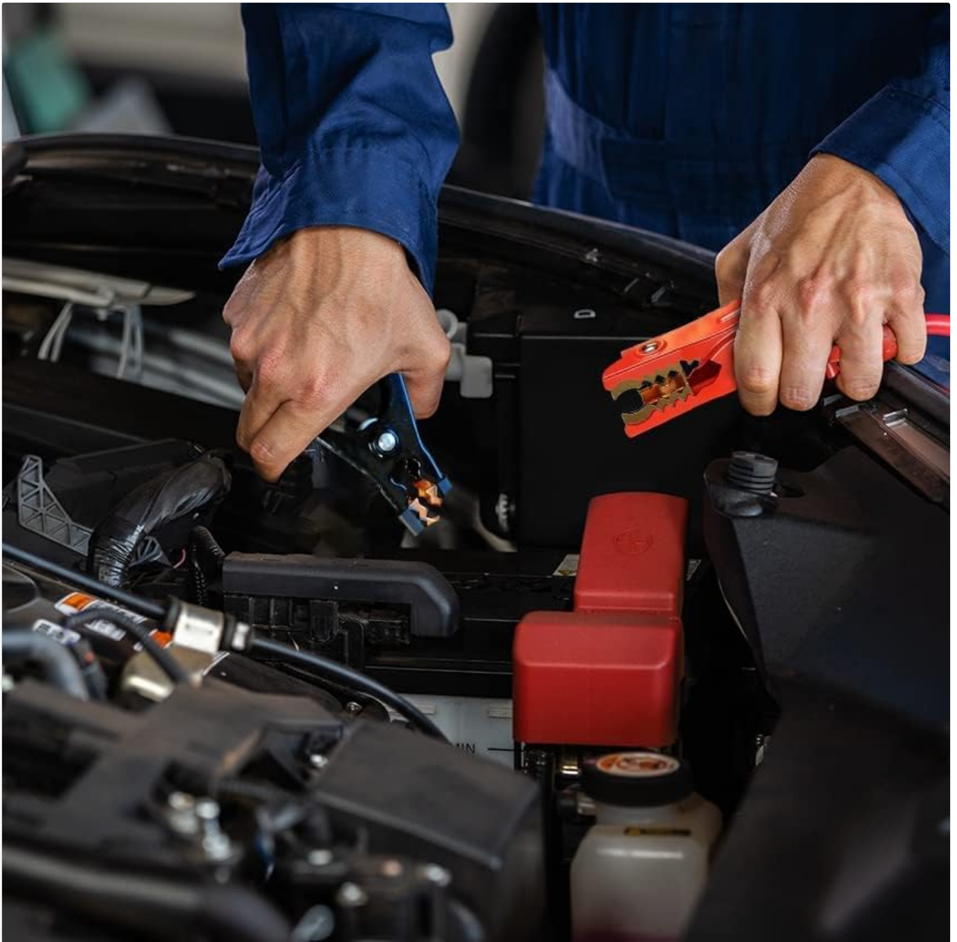
Image: A person's hands connecting a red jumper cable clamp to a car battery terminal, demonstrating the connection process.
