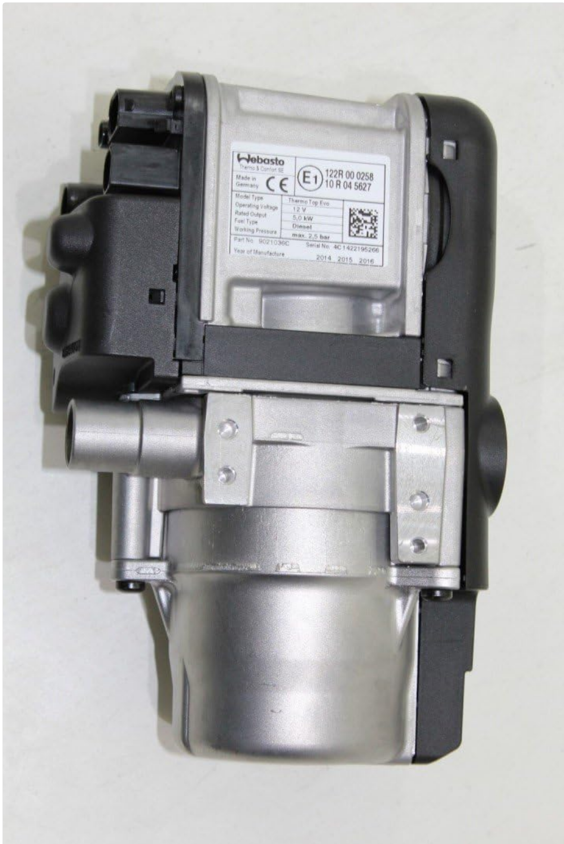
Image 2.2: Close-up view of the Webasto Thermo Top Evo 5+ heater unit, showing its compact design and connection points.
