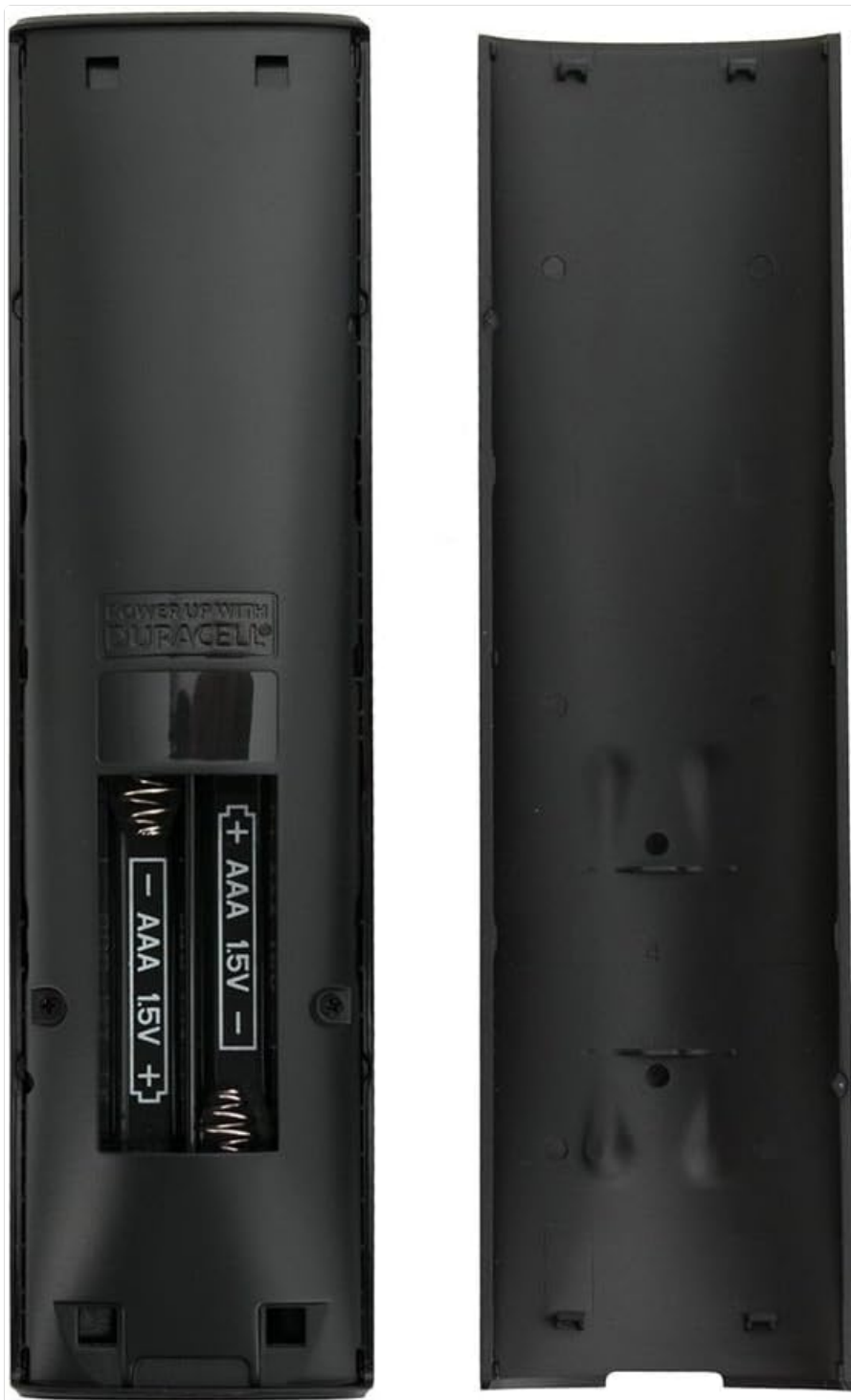
Figure 3.1: View of the battery compartment on the back of the XRT136 remote, indicating the correct orientation for AAA battery insertion.
