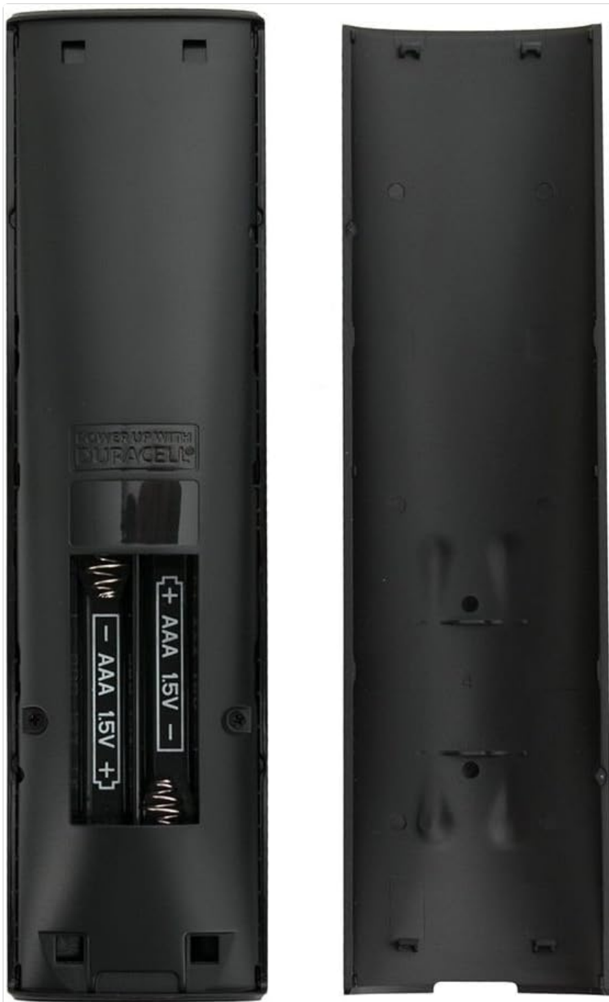
Image 3.1: Rear view of the USARMT remote control with the battery cover removed, showing the two AAA battery slots.
