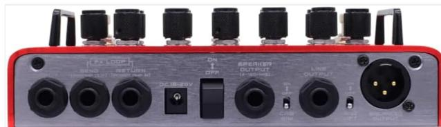
This image shows the rear panel of the Mojo Attack, detailing all available input and output connections.
