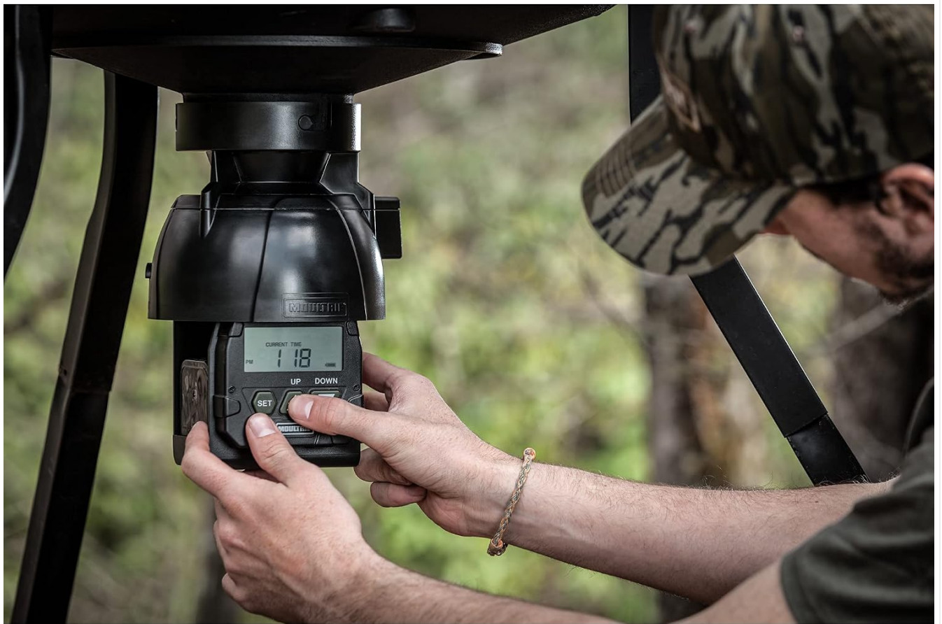
Figure 3: Programming the Easy Set digital timer.
