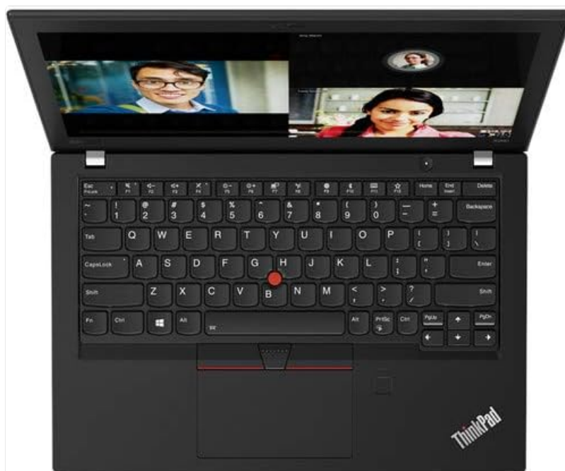
Figure 4: Keyboard and touchpad layout of the ThinkPad X280.
