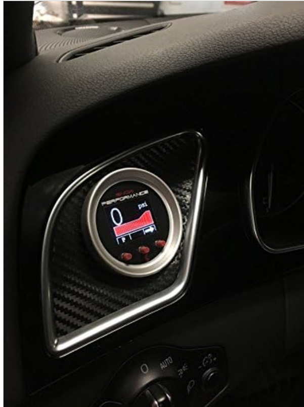
Figure 5.1: Example of the Snow Performance controller integrated into a vehicle's dashboard, displaying operational status.
