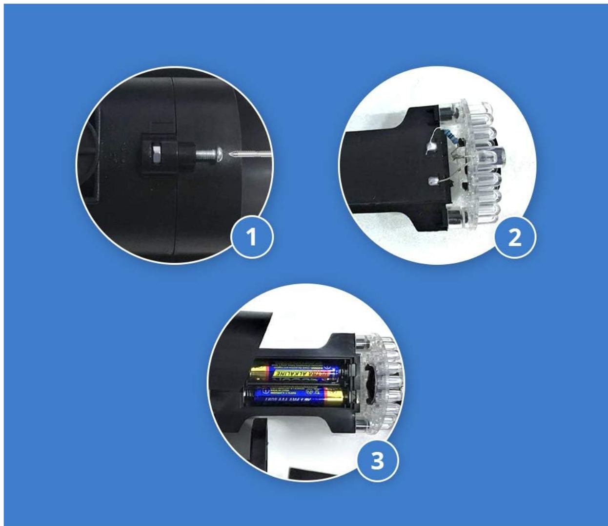
Image 3.2: Step-by-step guide for installing batteries into the dummy camera.
