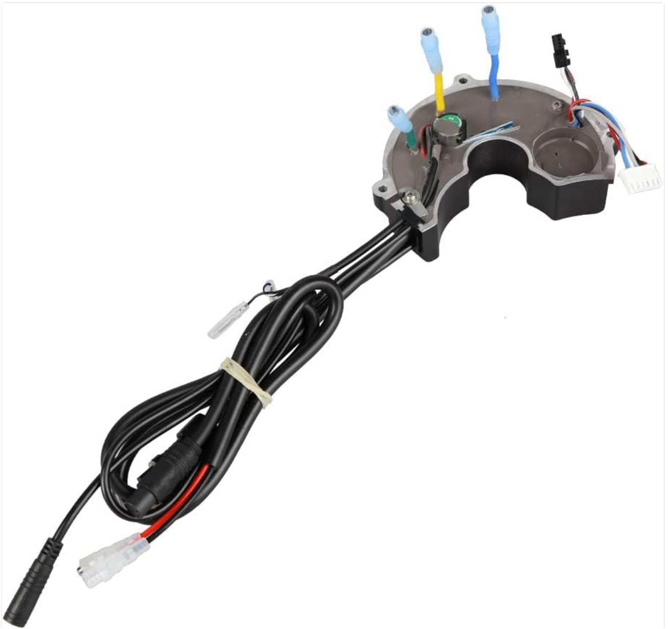
Figure 4.4: The BAFANG Mid Drive Controller with its cover removed, revealing the internal wiring and connections, which are crucial for understanding its functionality.
