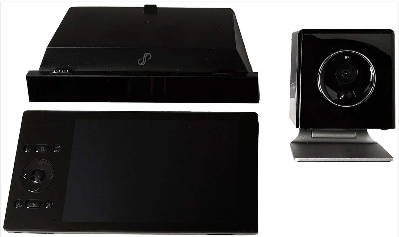
Figure 2.2: An overhead view of the Oomi FT101 components. From top to bottom: the main dock unit, the detachable Touch/Infinity display, and the Oomi Cube camera. This view highlights the separate nature of the components.
