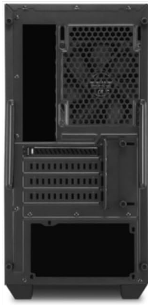
Figure 3: Rear view of the Sharkoon V1000, showing the I/O shield cutout, expansion slots, and power supply mounting area.
