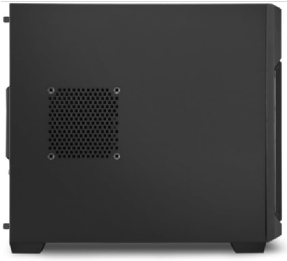
Figure 6: Side view of the Sharkoon V1000, showing the ventilation cutouts which may have associated dust filters.
