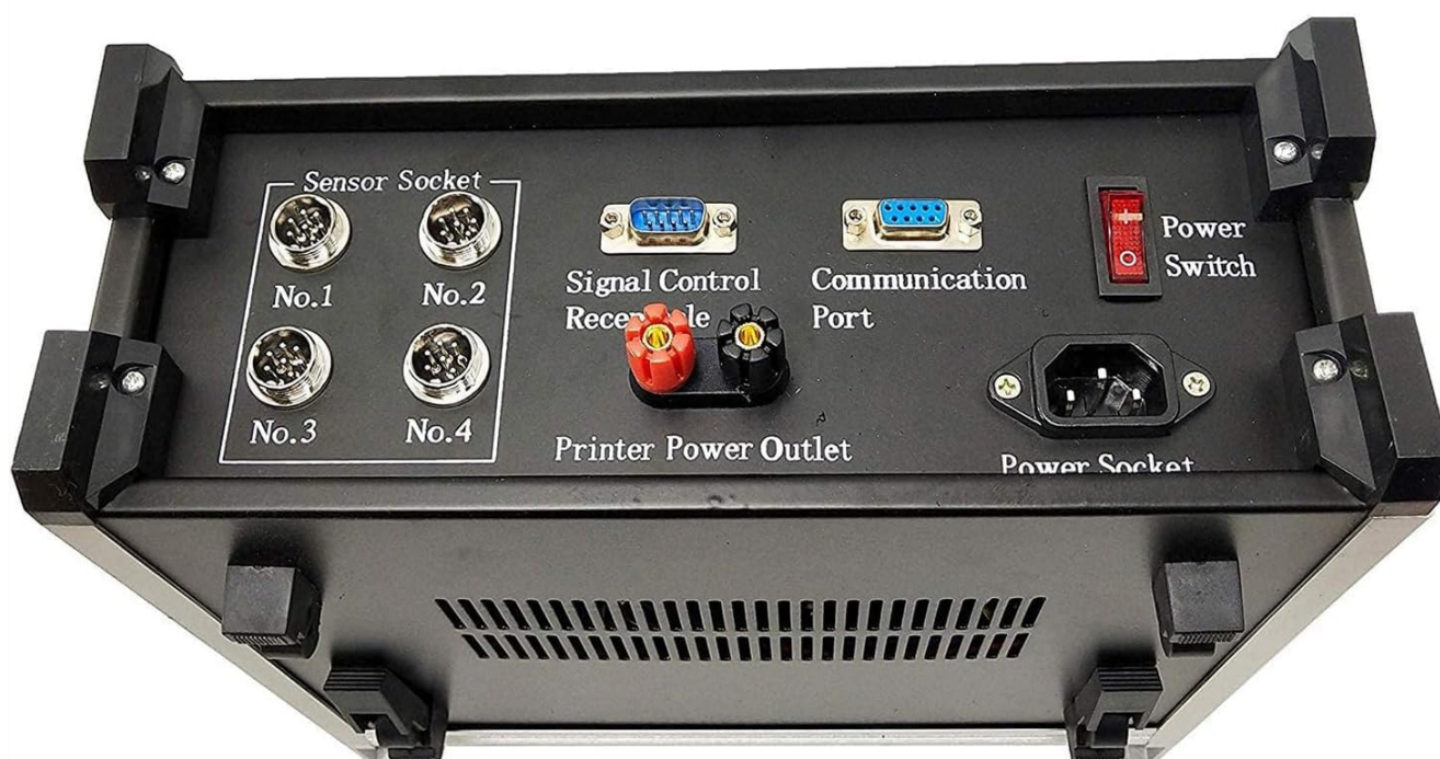
Image: The rear panel of the VD-99P meter, highlighting the sensor sockets, communication ports, printer power outlet, and power switch.
