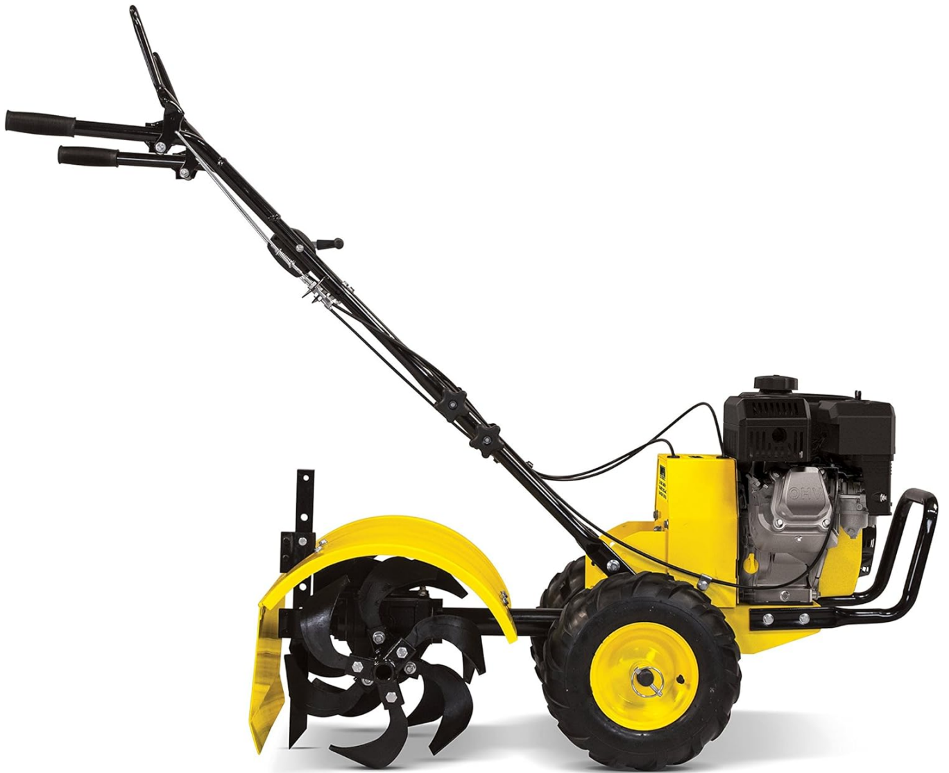
Figure 3.2: Side view of the tiller, showing the engine, handle assembly, and the rear tines with their protective shield.
