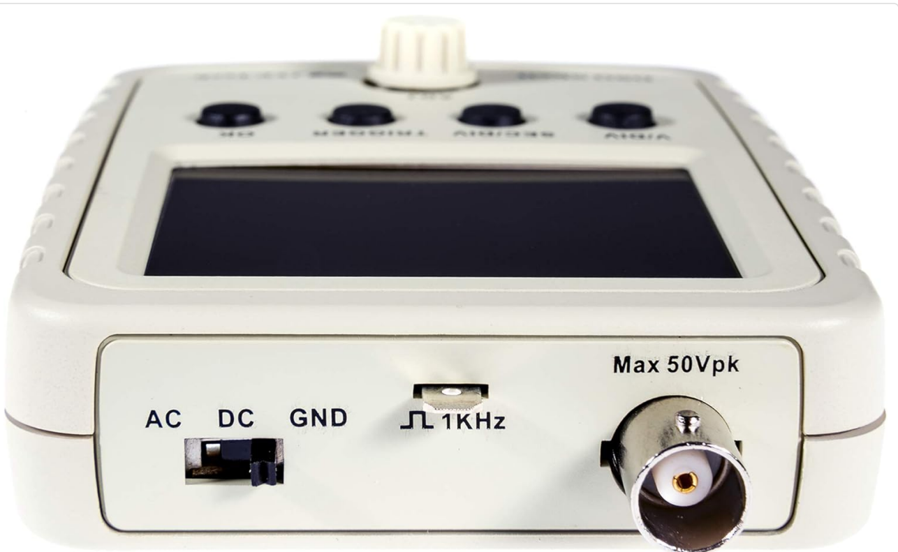
Figure 4: Top view of the DSO150, showing the BNC input connector, the AC/DC/GND coupling switch, and the 1KHz calibration output.
