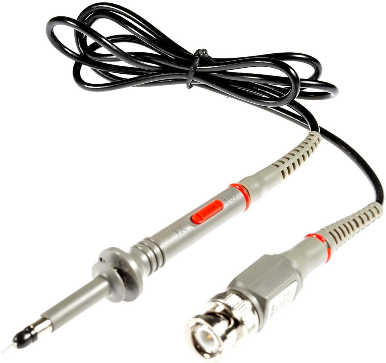
Figure 2: The included 1x/10x BNC oscilloscope probe, featuring a switch for attenuation selection and a BNC connector for attachment to the oscilloscope.
