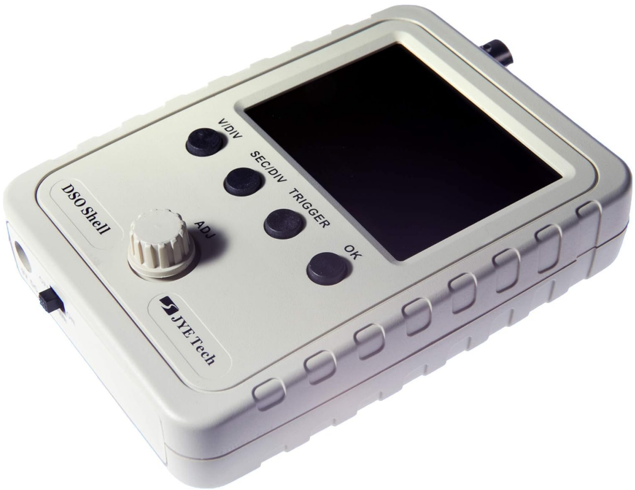
Figure 1: Front view of the DSO150 Oscilloscope, showing the display, control buttons (V/DIV, SEC/DIV, TRIGGER, OK), and the rotary adjustment knob (ADJ).
