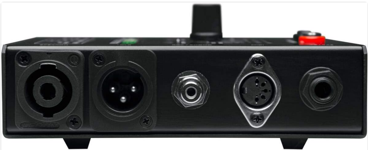
Figure 2: Top-down view of the Mackie MTest-1 Cable Tester, highlighting the diverse range of input and output ports available for testing.
