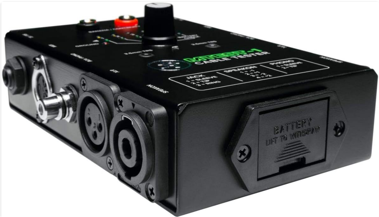
Figure 4: The Mackie MTest-1 with red and black continuity probes connected to the 'Banana / Continuity' jacks.
