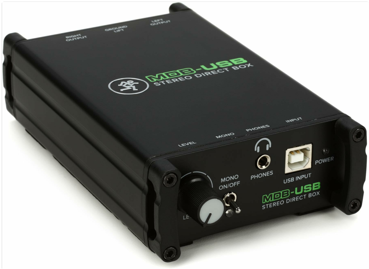
Figure 2: The Mackie MDB-USB's input and output panel, highlighting the USB input, XLR outputs, and headphone jack.
