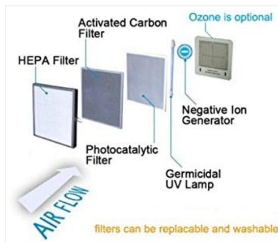
Diagram showing the air flow and the sequence of filtration components: HEPA Filter, Activated Carbon Filter, Photocatalytic Filter, Negative Ion Generator, and Germicidal UV Lamp. Ozone is an optional component.
