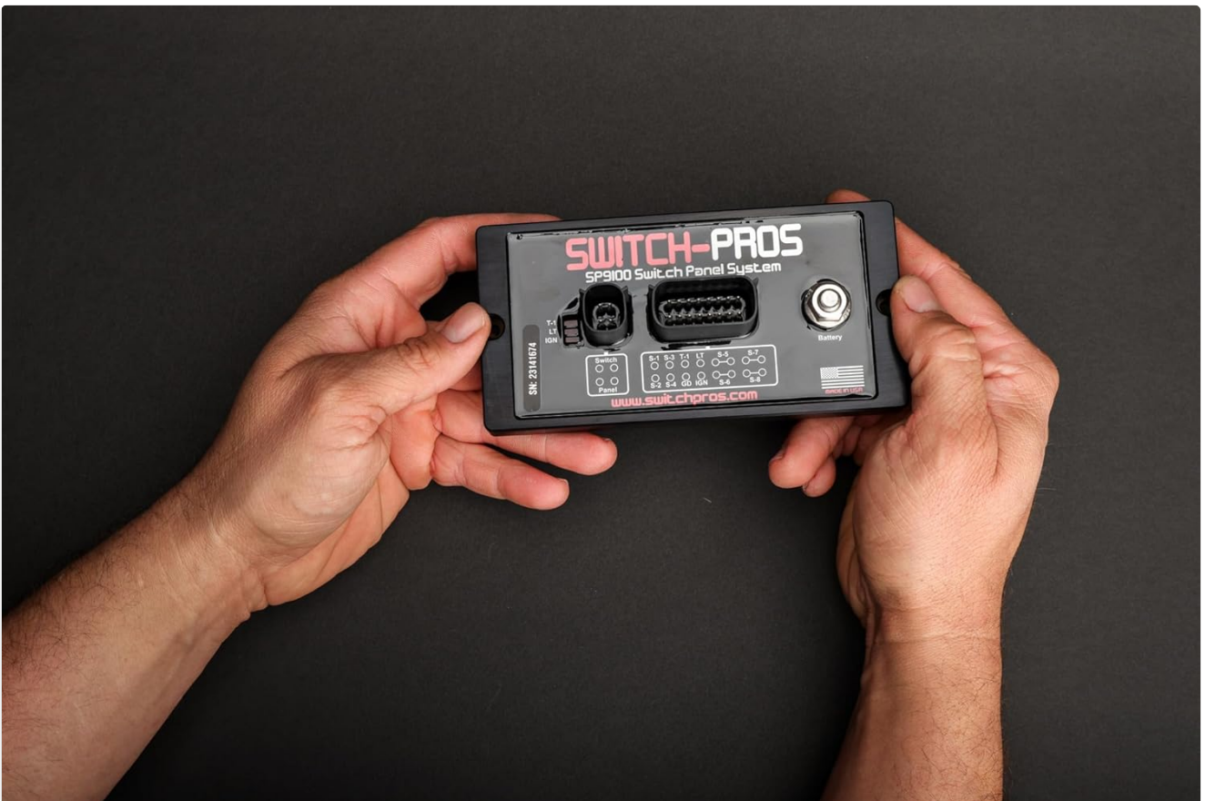
Figure 3: The SP-9100 power module, highlighting its input and output connections for electrical accessories.
