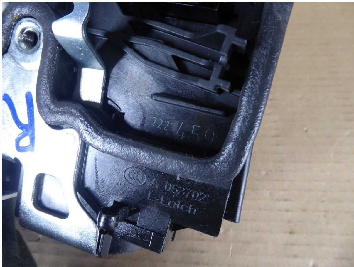
Figure 5.1: Detail of the electrical connector on the latch. This connector facilitates communication with the vehicle's central locking system and other electronic controls.
