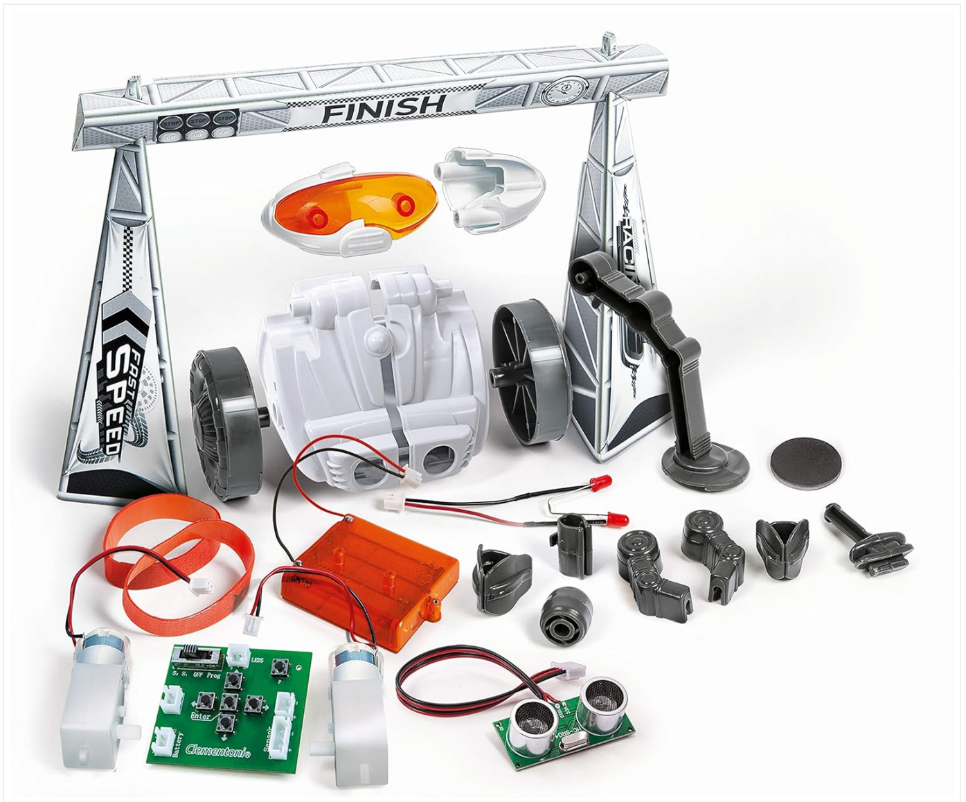
Image: All components of the Clementoni Galileo My Robot MC 4.0 laid out, including the main body, wheels, circuit board, motors, ultrasonic sensor, battery compartment, and various small parts for assembly.
