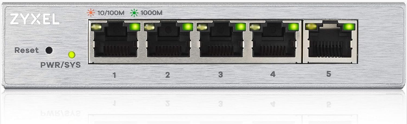
Figure 4.1: Front view of the Zyxel GS1200-5 switch, highlighting the five Gigabit Ethernet ports, the Reset button, and the Power/System LED indicators. The LEDs above each port indicate 10/100M (orange) and 1000M (green) link status.
