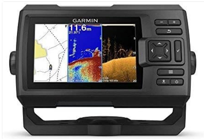
Image: The Garmin STRIKER Plus 5cv display showing a split screen with traditional sonar on the right and a mapping view on the left.
